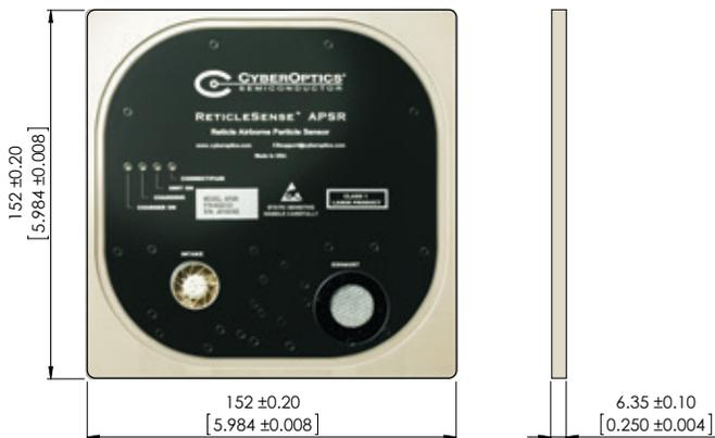
Dimensions, chamfers, and squareness conform to SEMI standard for 6 inch square reticles.
