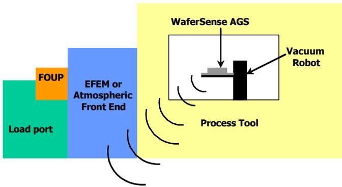
**Wireless Communication:** WaferSense AGS uses 2.4 GHz RF (Bluetooth®) wireless communication between the wafer and the link that is connected to a PC. WaferSense AGS uses a Class 1 Bluetooth device, rated for unimpeded communication up to 100 meters. Metal enclosures specific of a semiconductor use environment do not inhibit this communication.
