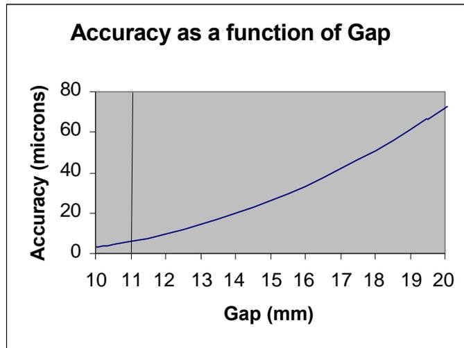
Films which may develop on the showerhead do not affect the capacitance significantly because they are thin relative to the total gap between the AGS and the showerhead. The effect of such films is smaller than the sensor accuracy. In practice, showerhead flatness issues tend to be larger than showerhead surface film issues.
