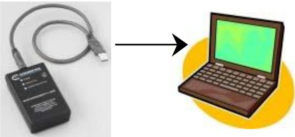
**Link & Laptop:** The link is a compact USB 1.1 compliant device that connects to a laptop to enable wireless communication with the teaching wafer.
