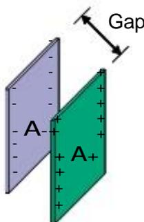
$$\text{Capacitance} = \frac{\text{Area} * \text{Dielectric Constant}}{\text{Gap}}$$
