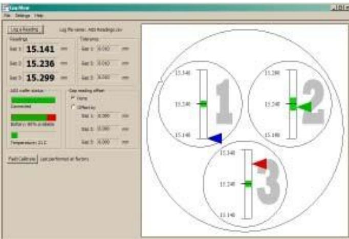
**GapView™ Software Application:** GapView displays numerical and graphical gap information. Each graphic is color-coded to make it easy to see whether it is above, below or within the selected target gap range.
