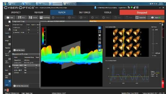
CyberCMM™, an extensive suite of CMM tools, provides 100 percent metrology-grade measurement on all critical points much faster than a traditional CMM, including coplanarity, distance, height and datum X, Y, to name a few. A fast and easy setup can be performed as compared to a slow, engineering resource-intensive setup that typically requires multiple adjustments with traditional CMMs.
