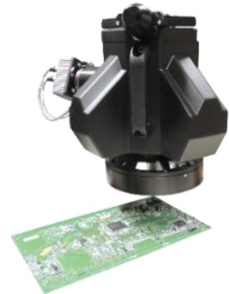
Also on display, the QX250i™ simultaneous double-sided AOI system offers fast, flexible and high performance inspection for all applications, and is ideally suited for pre-reflow and selective solder inspection. The top and bottom high-resolution Strobed Inspection Modules (SIMs) with enhanced illumination provide a single platform for the inspection and defect review process that shortens the production line and drives approximately 50 percent productivity improvement.
