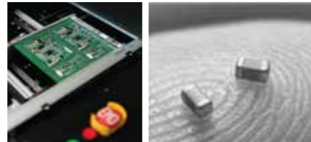
01005 component size inspection capability
